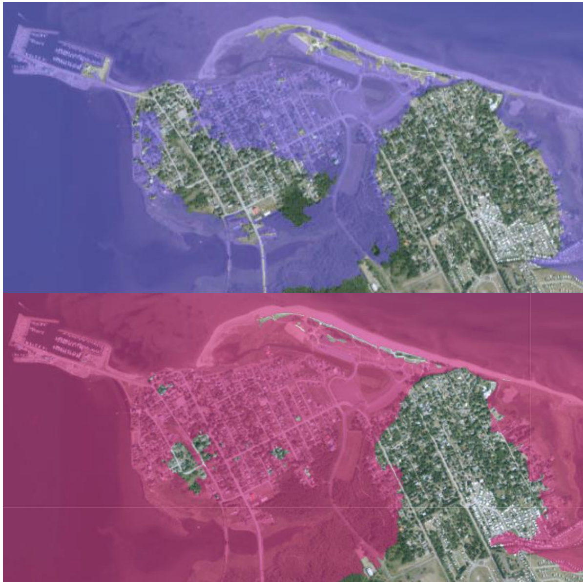
Figure 5-1: Project flood extents during Present-Day, 1 in 100-year event (Top, blue shaded area) and 2100, 1 in 100-year event (bottom, pink shaded area) (Source: Service New Brunswick, 2022)
